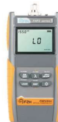
Part Number Description FHP2B04 Optical power meter, 850/1300/1310/1490/1550/1625nm, FC/PC connector, -50 to +26dBm, with USB, data storage and wavelength recognition functions
